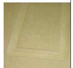
▲ The MDF Sealer ensures dimensional stability and protect edges and milled grooves against absorption of moisture
