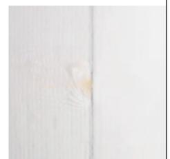
▲ The white-coated pine on the left was treated with a conventional primer while on the right it was coated with Teknos' knot sealing primer
